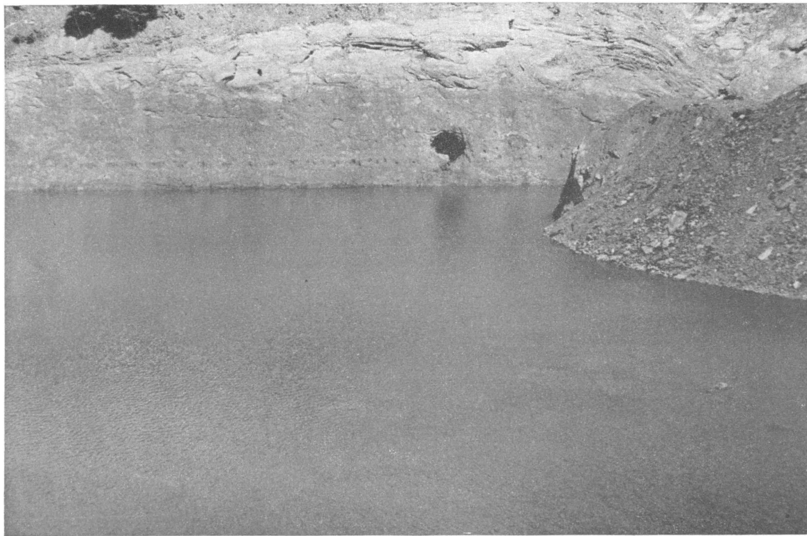
FIGURE 46.—Holmes Pocket stripping, near Tuscarora, showing underground tunnel discharge into pool, Southern field.
