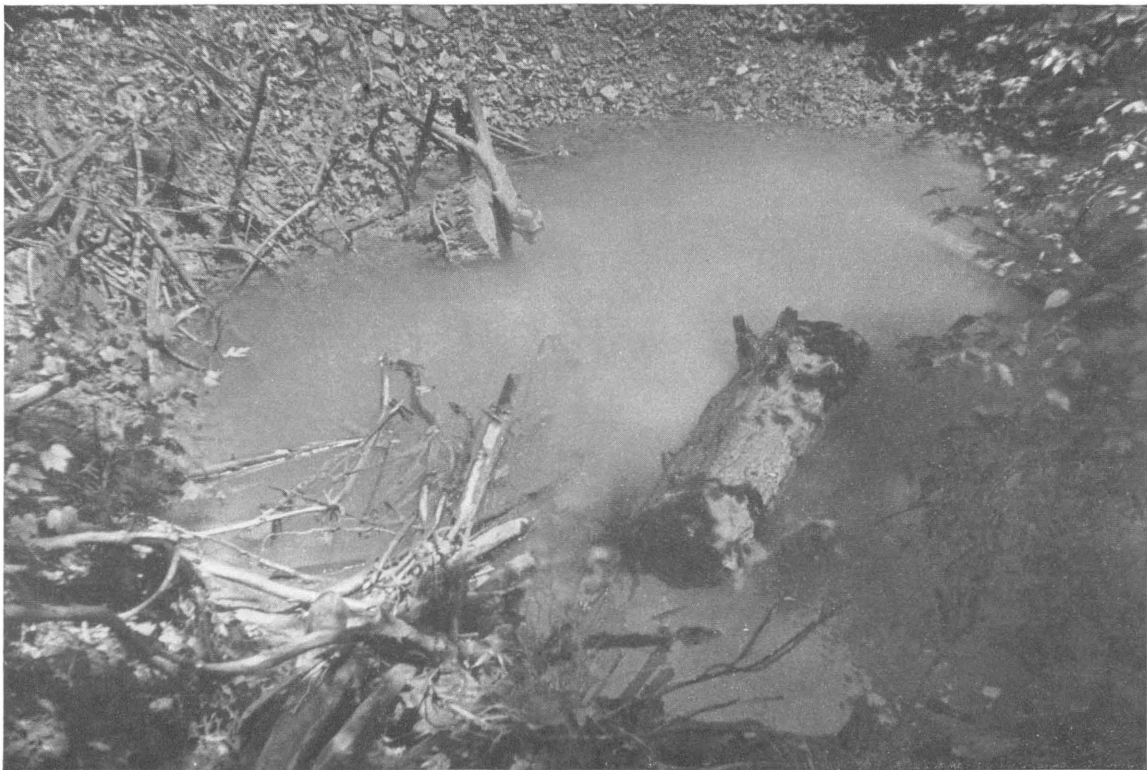
FIGURE 50.—Underground water pool overflowing to surface through outcrop fall at Mary D colliery, Southern field.
